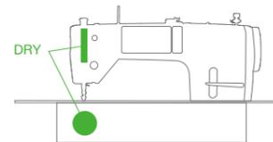
• The section around the needle bar, the thread take-up lever and the hook are not lubricated.
