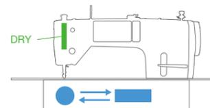
• The needle bar and thread take-up components are not lubricated.
