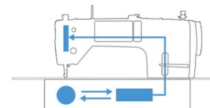
• The needle bar and thread take-up components are lubricated with the minimum required quantity of oil. For the hook section, the standard method of lubrication is employed.
