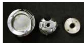
The non-rotary bobbin eliminates irregular stitches which have a tendency to occur at some sewing speeds and bobbin-thread tension fluctuations which have a tendency to occur according to the bobbin thread remaining on the hook. Since the bobbin thread is fed without rotating the bobbin, the bobbin never idles.
