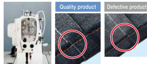
**The active presser foot pressure mechanism demonstrates its effectiveness in prevention of stitch gathering and loose stitches.**
