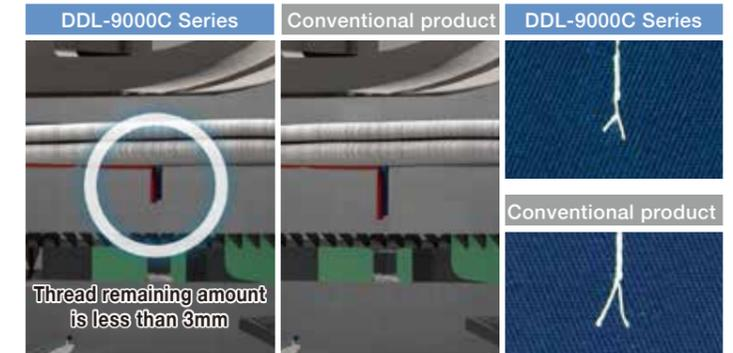
Thread remaining amount is less than 3mm
